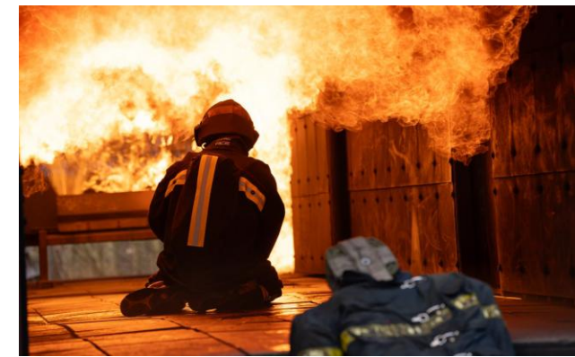
Testing of the firefighter's poncho and suit in the Flashover Container (FOK) in Zbiroh.
