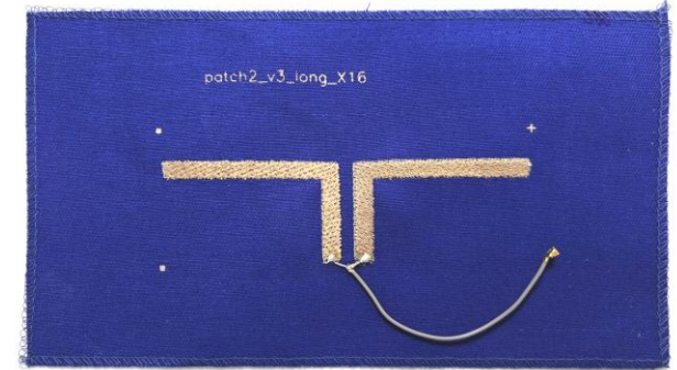
Textile dipole antenna with hybrid construction antenna
