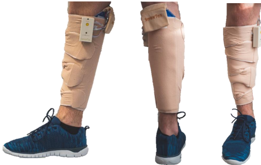
The final functional sample of a smart sleeve for edema monitoring on the proband's leg.
