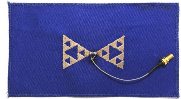
Textile bowtie antenna with hybrid construction bow-tie
